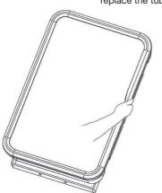
Push the rubber ring aside and remove the screws at backside, then take out cover.
